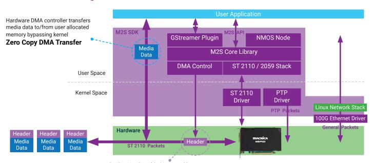
Packet Header added/removed by ST 2110 IP FPGA HW Engine
